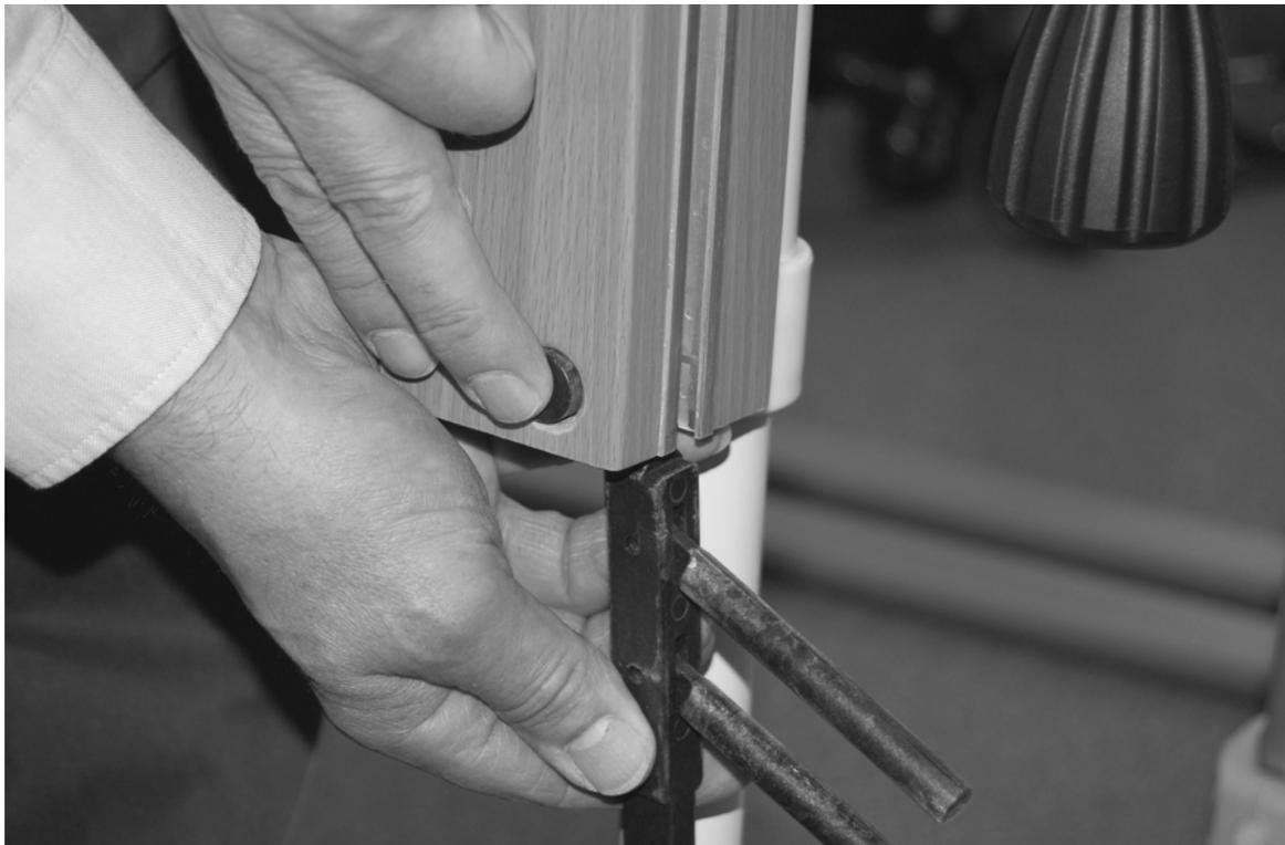
Fully insert the slider (pointed end up) until it locates in its lowest position. Fit both side rails to the slider with the rounded edge to the top. The other ends of the rails should rest on the floor. (see following images)
